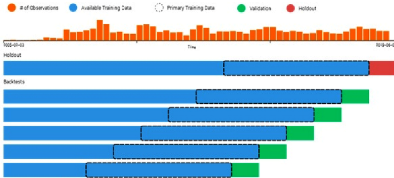
Figure 5.6. Illustration of out-of-time validation (OTV). For a color version of this figure, see www.iste.co.uk/jurczenko/machine.zip
