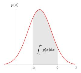
Our aim is to calculate the probability that X takes a value between two positive numbers 'a' and 'b' where b>a. The shaded area under the curve represents that probability.
