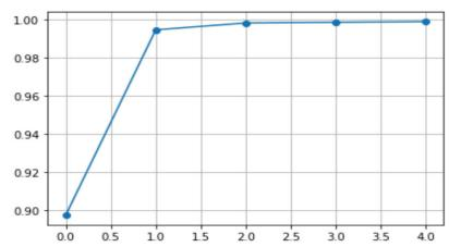
**Observation -** We can see that out of the 30 components, the four most significant ones can explain almost 100% of the variance.
