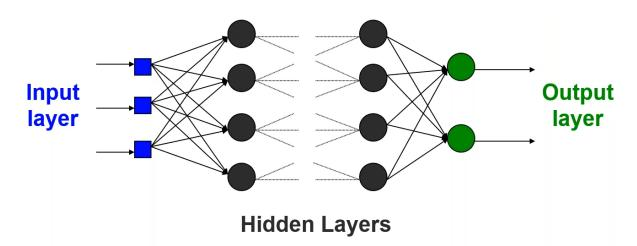
The architecture is as follows. Each circle, as described above, can be interpreted as a neural network. There are 3 layers. First, we have the inputs, then we use these inputs to get signals with the hidden layers. This intermediate layer then gives a result, the output layer, which can be a prediction of a stock price movement based on OHLC data (input data).
