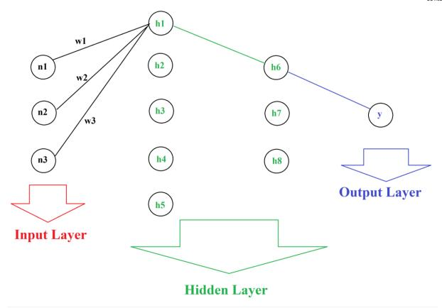
In the input layer, you have the inputs, each input "n", will have its unique weight "w". The product of each input together with its weight the corresponding sum of all of them makes the  $\Sigma$  model.
