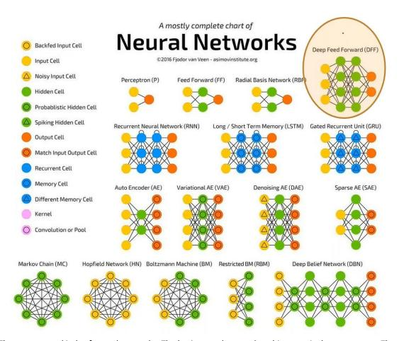
There are many kinds of neural networks. The basic neural network architecture is the perceptron. The perceptron (P as in the figure above), consists of only an input and output layer. In the input layer (yellow circles), you will find
